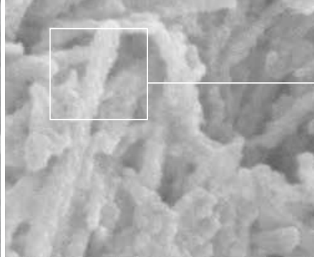
Densely packed calcium fluoride-like particles after the application of Fluor Protector S, Scanning electron micrographs, magnification: 30'000 x (Ivoclar Vivadent, R&D 2012)
